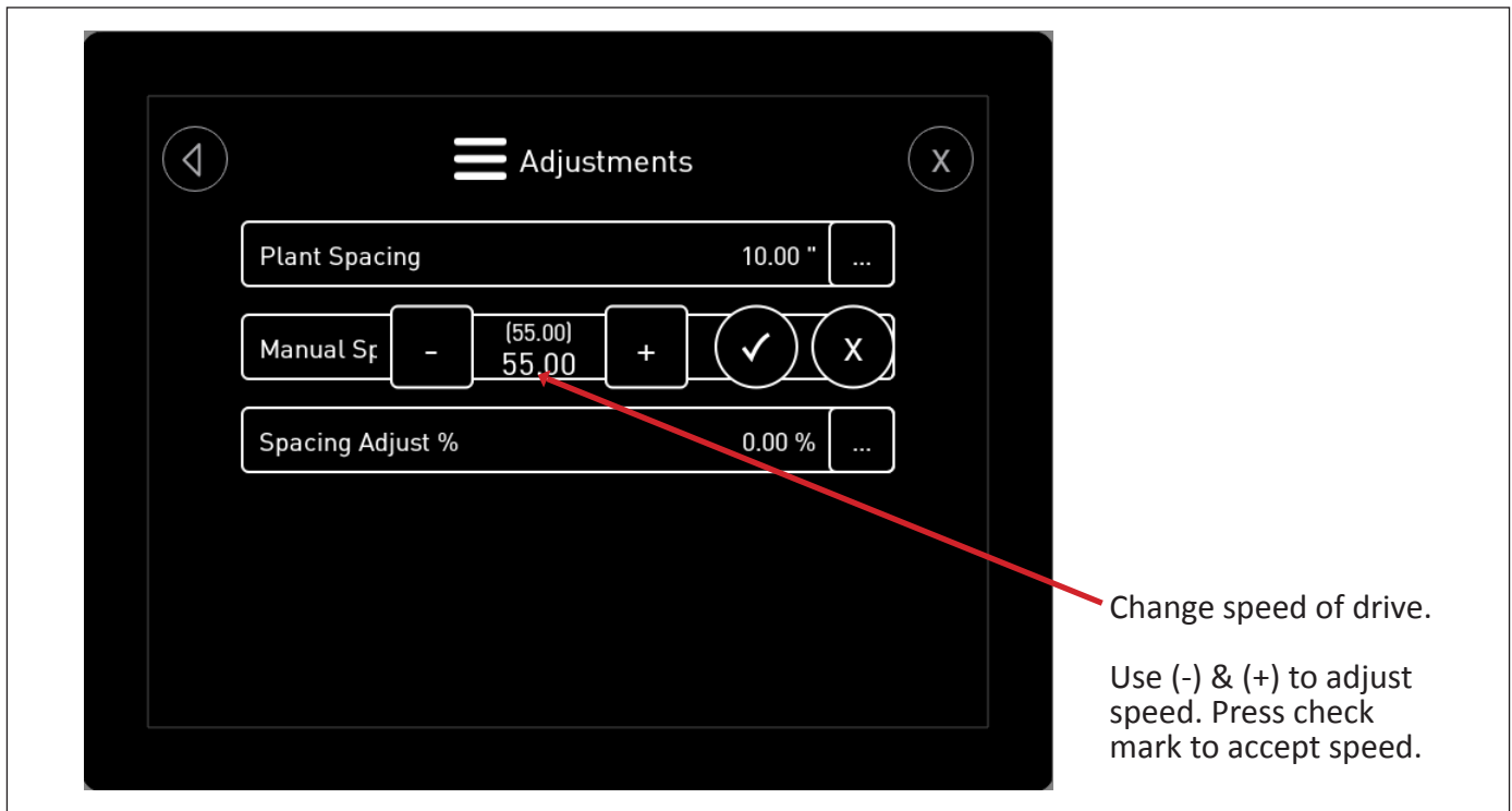
Fig. 45 Screen Operation - Manual Spacing Adjustments
